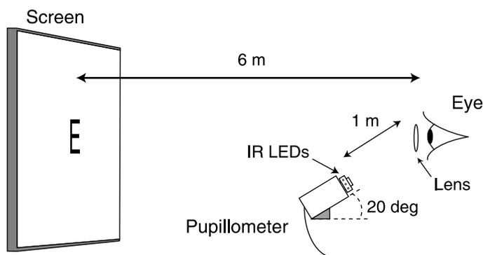
Figure 1. Setup for the simultaneous visual acuity tests and pupil diameter measurement.
