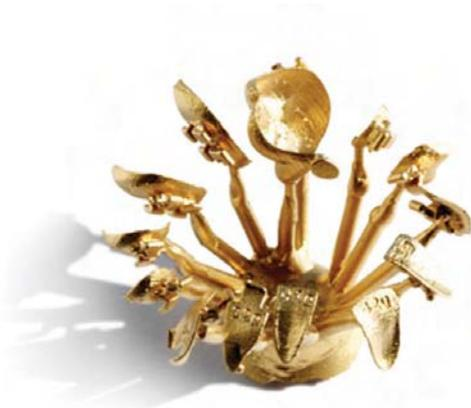
FIGURE 8: The final brackets after investment casting.
