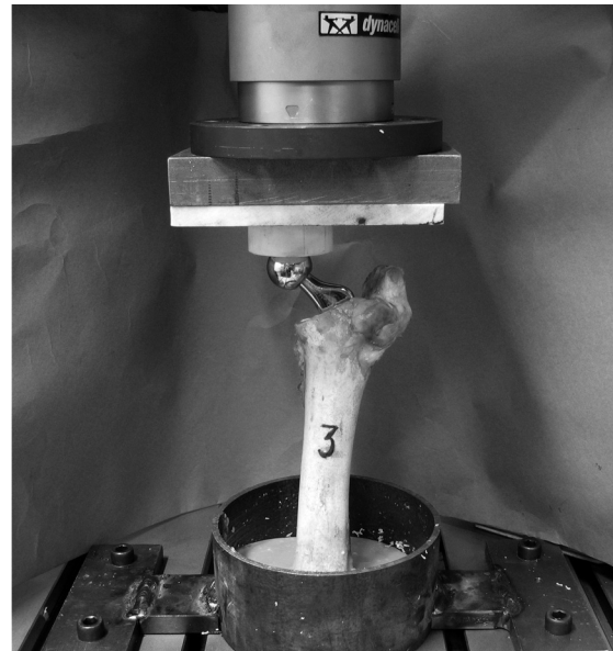
Figure 3. Axial cyclic loading between 440 N (swing phase of gait) and 1,320 N (stance phase of gait) through the 28-mm femoral head, by direct contact with the hydraulic fatigue testing machine via a PTFE disc, which was free to slide along a PTFE plate.
